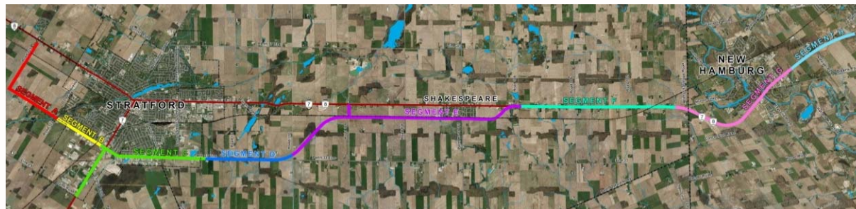
Segment G: 6-lane cross-section with 7 m median from west of Peel Street to east of Hamilton Street intersections
