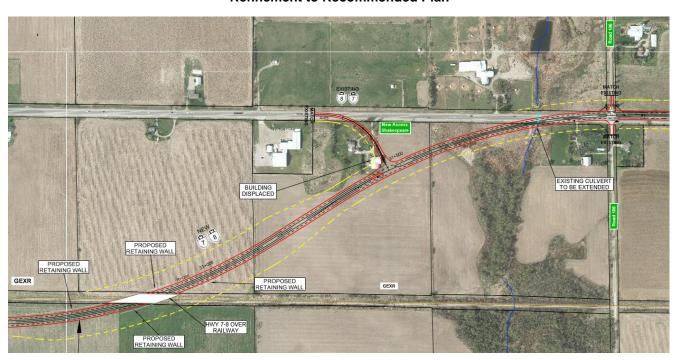
Road 109 intersection treatment at new Highway 7&8 crossing and existing Highway 7&8 connection:
