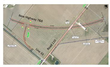
The existing Highway 7&8 alignment east of Shakespeare has been refined to allow for the provision of a full moves intersection between existing Highway 7&8 and New Highway 7&8 west of Road 106 (east of Shakespeare), addressing emergency response concerns and providing improved access to / from Shakespeare.
