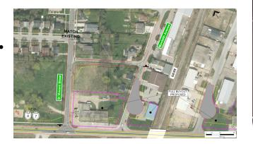
Line 33/Road 110 Intersection: The existing Road 110 alignment will be retained, crossing over New Highway 7&8, with access to New Highway 7&8 provided via Line 33. The Line 33/Road 110 intersection will accommodate all movements. This revision results in reduced property requirements and reduced impacts to the agricultural lands while maintaining the local road network continuity.
